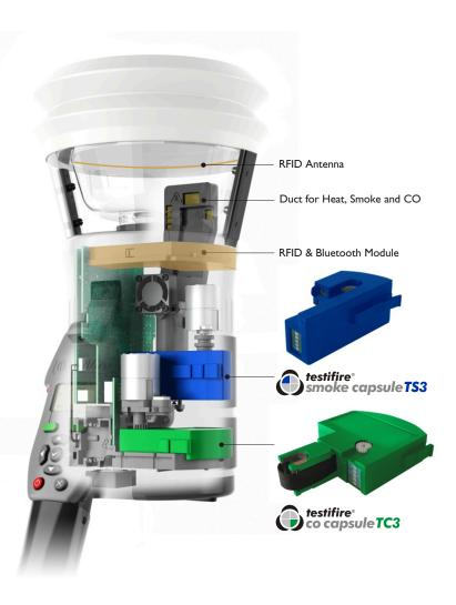
Smoke, Heat and CO stimuli are created in a single test unit, and delivered individually, or - for the first time - simultaneously, in whichever combination is required. Testifire does this without using pressurised cans of gas or hazardous media. Stimuli (Smoke, Heat, and CO) are generated at the time of test using safe and patented processes fuelled by replaceable capsules.
